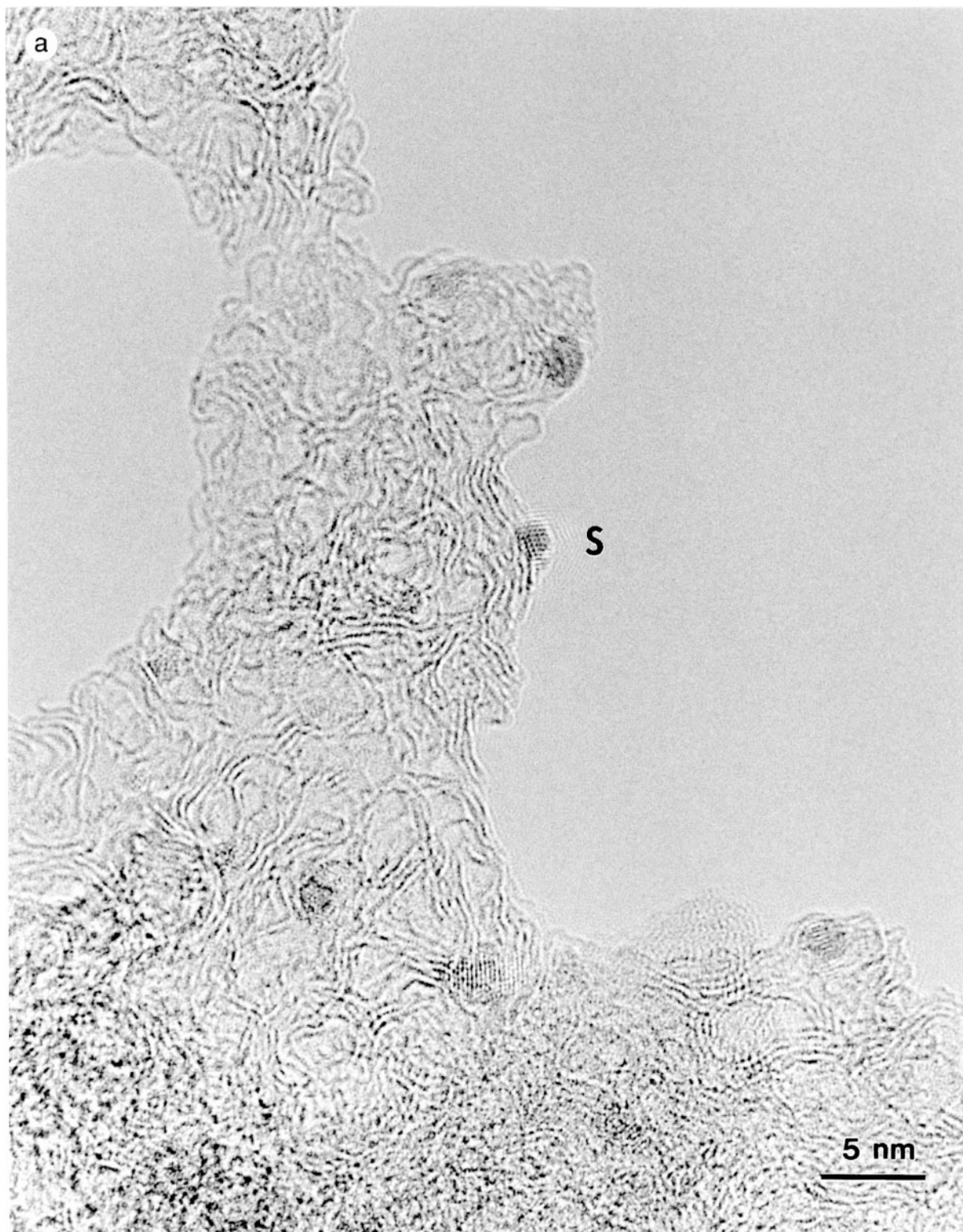
FIG. 4. (a) A TEM photograph on Rh(C)/AC (2 wt%) with CO treatment at 473 K after the H 2 treatment; (b) an energy-dispersive X-ray spectrum on the spot shown in (a).
